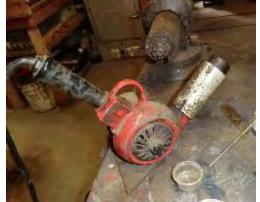
Because of the use of a venturi burner (as opposed to Don's design which uses a blown system), a tiny blower is needed. Without the blower, the pressure in the forge is sufficient to choke the burner. The blower is a 12V squirrel cage and plugs into the bell of the burner. The system needs only 3 to 5 psi to hover at 1550 F and reaches that temperature in about 15 minutes from light off.
